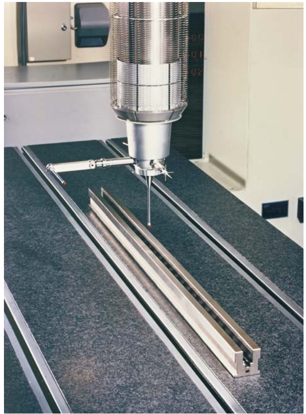
Fig. 8: KOBA-step aligned along the X-axis (lying flat on the table with no accessories used), stylus probe vertical.
