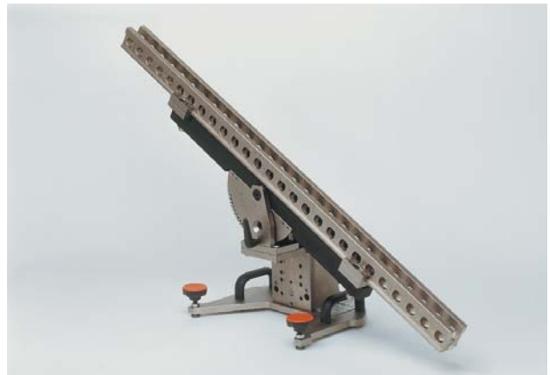
Fig. 14: KOBA-step, equipped with swivel support base Size 1 for accommodating 1020 mm length step-gauge (stylus probe not shown).
