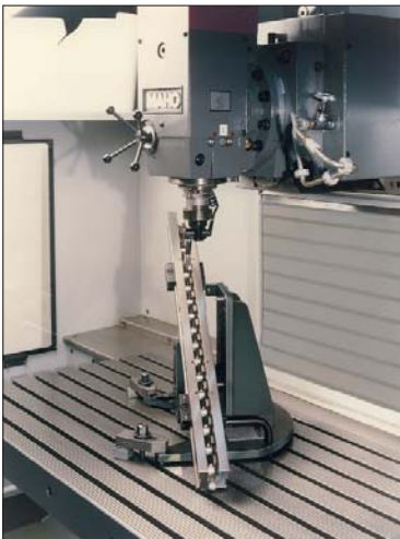
Fig. 15: KOBA-step installed on a swivel support and base, shown here spanning the major diagonal of the workspace of a vertical milling machine equipped with a dimensional-gauging head.
