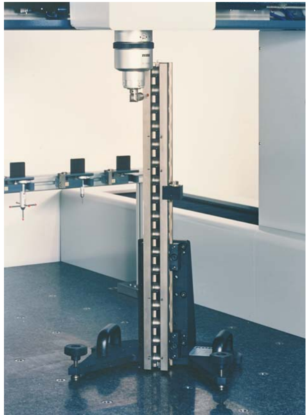
Fig. 10: KOBA-step aligned vertically along the Z-axis (standing in the base), stylus probe horizontal.
