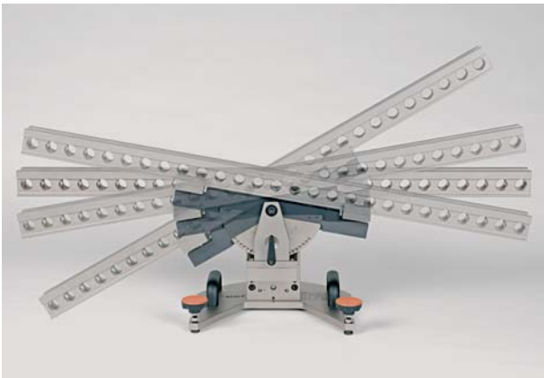
Fig. 13: KOBA-step with swivel support and base, illustrated at various angular inclinations (stylus probe not shown).
