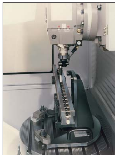
Fig. 18: KOBA-step, shown here installed on a flexible machining center for verifying its positioning accuracy (the center's dimensional-gauging head is integrated into its tool chuck).
