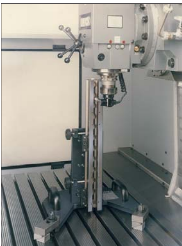
Fig. 17: KOBA-step, shown here aligned vertically for checking the Z-axis of a machine tool equipped with a dimensional-gauging head.
