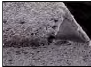
Diamond Delamination (Note: Large Grain Size)
