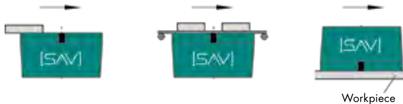
Use of table demagnetizers
