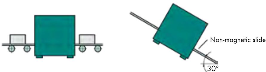
Tunnel demagnetisers with belt conveyor and slide
