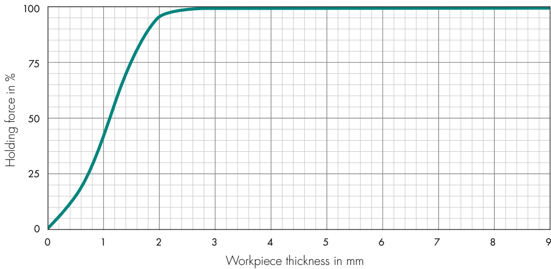
SAV 244.73 min. thickness of workpiece for circular magnets with fine parallel pole pitch 4 mm
