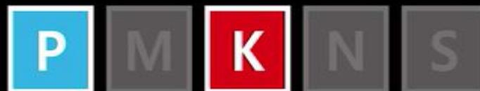
**Carbon steel / Alloy steel / Cast Iron**
